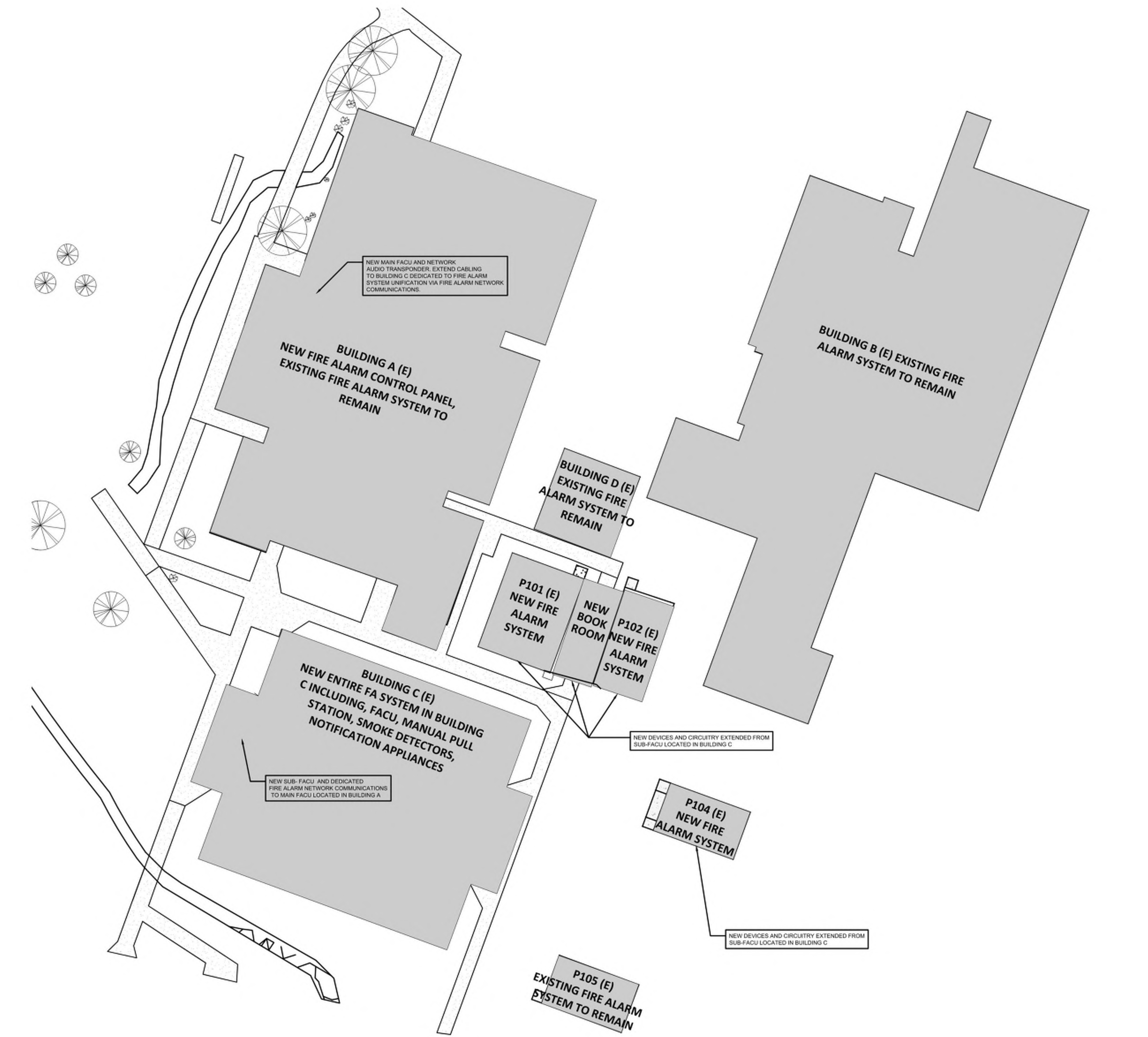
1 FIRE ALARM NEW SITE PLAN 1" = 20'-0"
